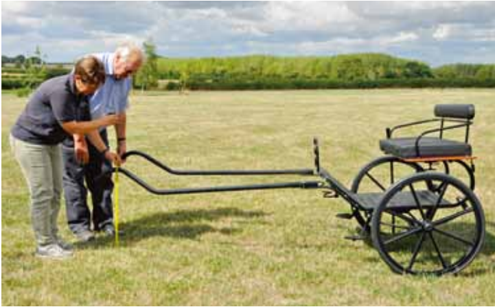
On most two-wheelers, the shafts can be adjusted on a series of holes to raise/lower the shaft height, or for fine adjustment the tugs can be moved on the back band
