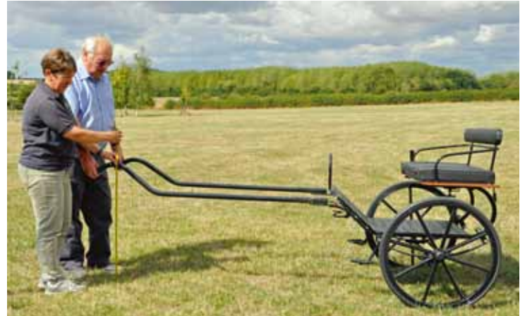
To achieve the correct balance (i.e. the shafts floating in the tugs when being driven) in a two-wheel carriage the floor should be horizontal to the ground
